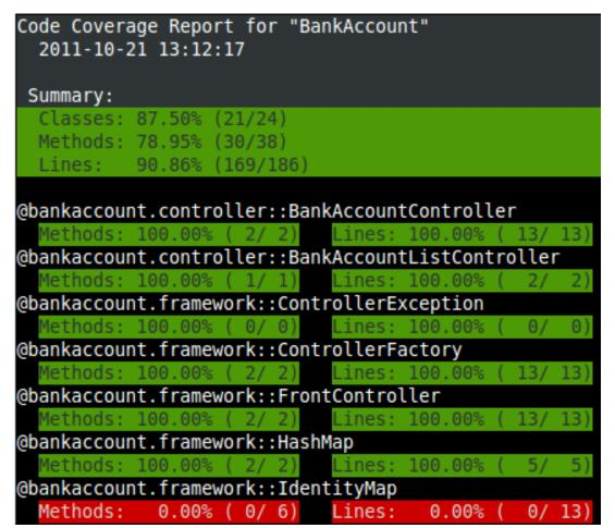
Figure 18.1. Code Coverage output on the command-line with colors
